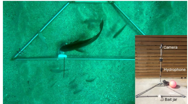
FIGURE 1 Baited underwater video (BUV) deployed in 5 m water in the marine reserve. Snapper are shown near the bait jar. Insert shows photograph of BUV. The triangular base measured 1.7 \text{ m} \times 1.2 \text{ m} \times 1.2 \text{ m}
