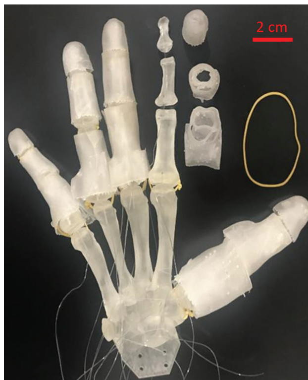
Figure 1. Major materials and components of our robotic hands. Soft and stiff 3D printing materials were used for producing the tissues and bones, respectively. Nylon cables and rubber bands were used for simulating tendons and ligaments.
