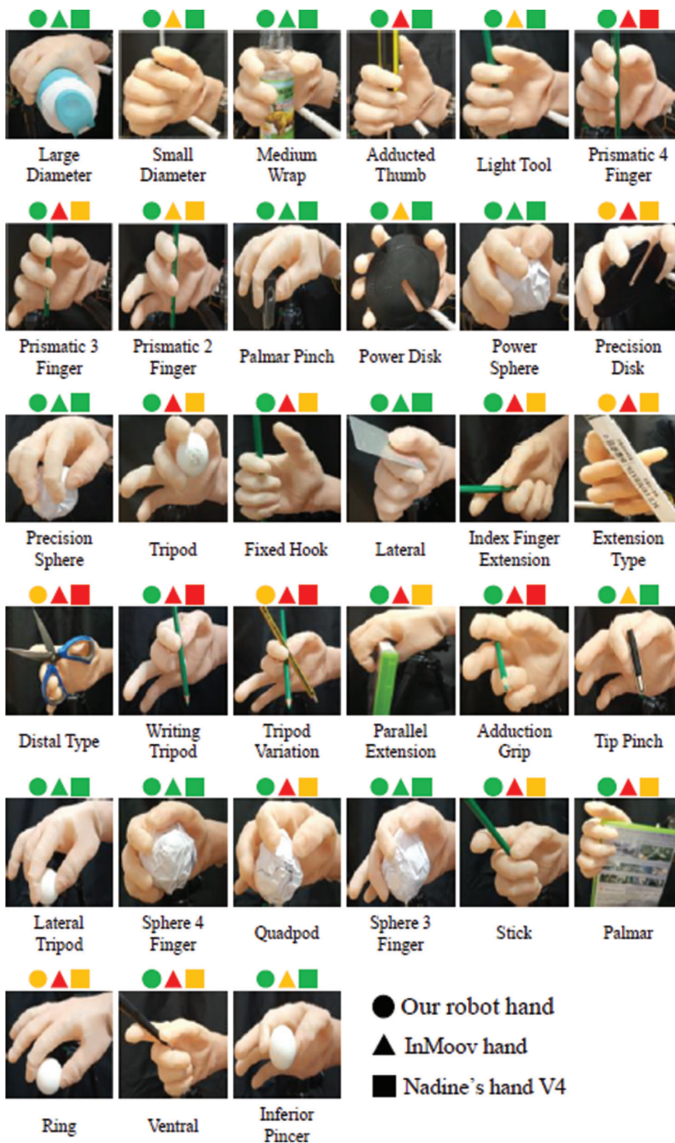
Figure 5. Comparison of object grasping success rates of different methods. Methods with success rates \geq 0.8 , in [0.2; 0.8) and < 0.2 are labeled in green, yellow and red, respectively. The proposed robotic hand has the highest success rates for all grasping gestures.
