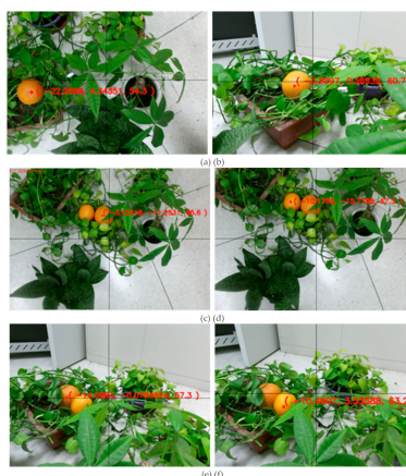
Figure 12. Partial representative results of crop feature point location experiments. (a) and (b) indicate the feature point location result when there is only one crop; (c) and (d) indicate the location of the feature points when there are two crops that are not occluded from each other; (e) and (f) indicate the feature point location results for two partially occluded crops.
