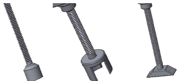
FIGURE 5: Different bottom connections of the prosthesis.
