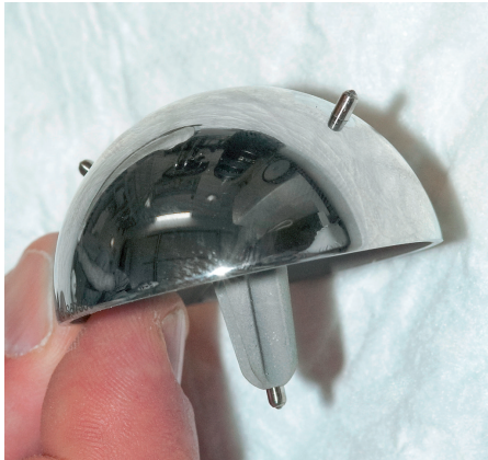
Figure 1. The Copeland humeral resurfacing head used in the study. The implant has been modified for standard RSA with 3 tantalum markers (arrows).
