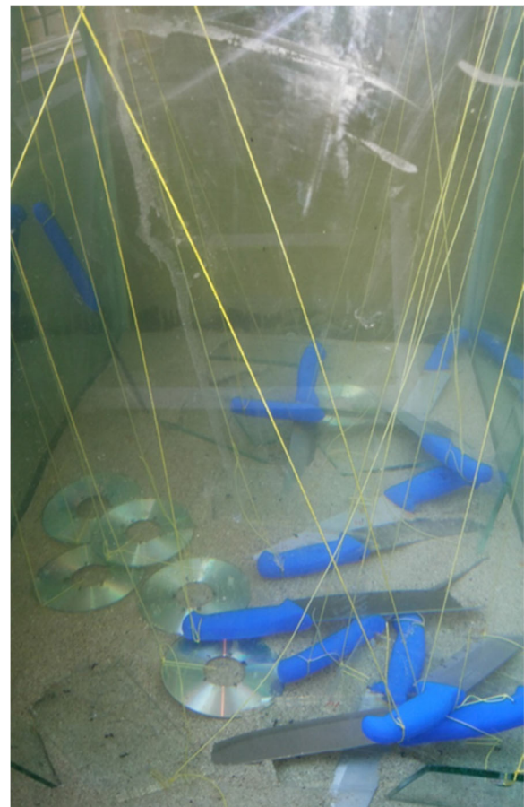
Fig. 1 non porous surfaces were placed in aquarium tank filled with type of water of study after fingerprints deposition
