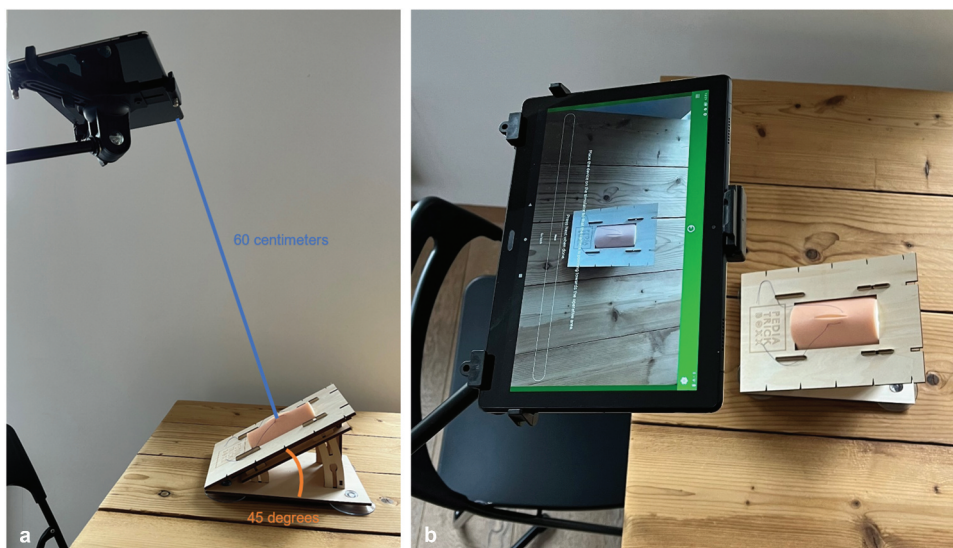
Figure 1. a and b Research setup with a Lenovo P10 tablet in a stand and a simulator by PediatricBoxx.
