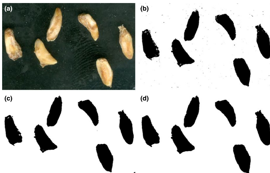
FIGURE 2 Schematic view of preparing images to determine the morphological parameters of VJG cultivar (a=original, b= make binary & threshold (Autso), c=median filter ( r = 2 pixel), d=dilation)
