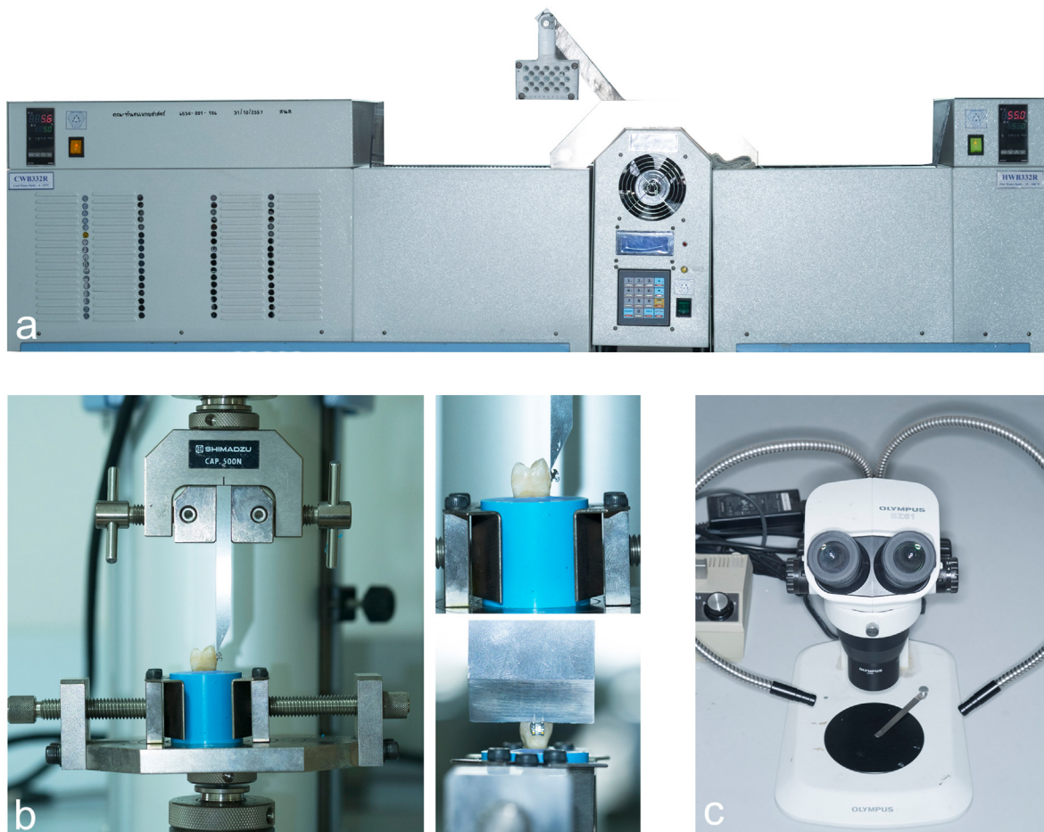
Figure 2. The machines used in this study, (a) the thermocycling machine, (b) the SBS test using the universal testing machine, and (c) the ARI score evaluated under the stereomicroscope.
