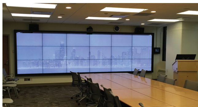
Figure 1: Tiled display with scalable adaptive graphics environment in the UIC pathology informatics learning and innovations laboratory
