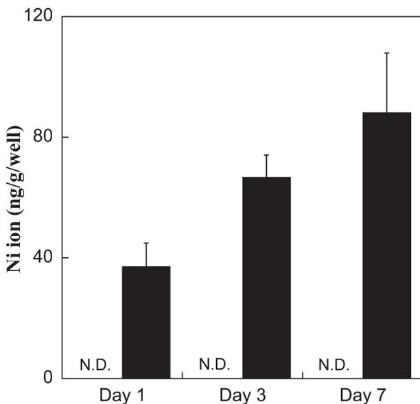
**FIGURE 3.** Concentration of Ni ions eluted from HNS (gray bar) and SUS316L (black bar) after immersion in PBS at 37°C for 1, 3, and 7 days. Data are the average  $\pm$  SD of five samples. N.D. means not detected.
