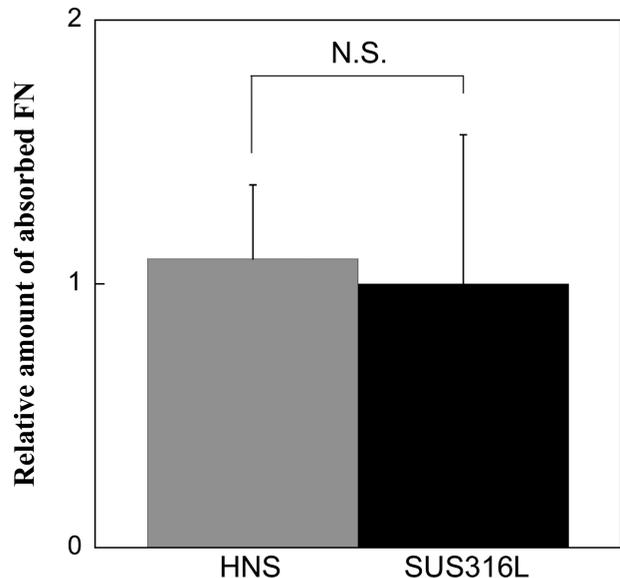
**FIGURE 2.** Relative value of adsorbed FN on the surface of HNS (gray bar) and SUS316L (black bar) assuming that SUS316L is 1. Data are the average  $\pm$  SD of five samples. N.S. means no significant difference.
