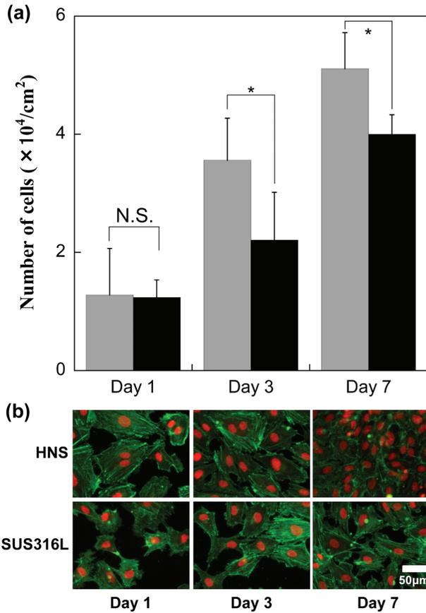
**FIGURE 1.** Endothelialization property of HNS and SUS316L. (a) Number of HUVECs on HNS (gray bar) and SUS316L (black bar) after cultured for 1, 3, and 7 days. Data are the average  $\pm$  standard deviations (SD) of five samples, with (\*) indicating  $p < 0.05$ . N.S. means no significant difference. (b) Distribution and morphology of HUVECs on HNS and SUS316L after cultured for 1, 3, and 7 days. Actin filaments (green) and cell nuclei (red) are shown.
