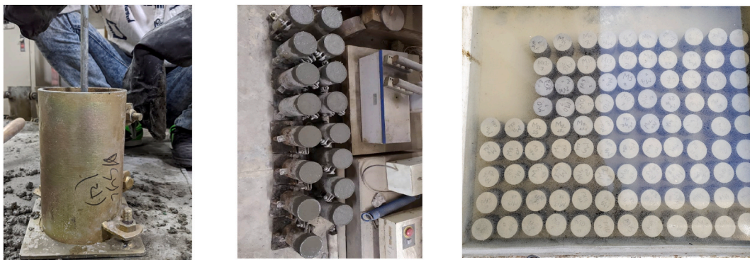
Fig. 2. Preparation and curing of the concrete cylinder specimens.
