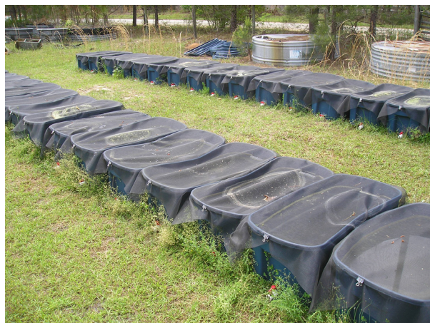
Figure 2. Photograph of the experimental setup. Mesocosms consisted of thirty-six 189-L plastic containers with overall dimensions of 108 cm × 55 cm × 45 cm arranged in two rows of eighteen. Mesocosms were covered with screen and had drainage valves installed near the bottom to manipulate water levels.
