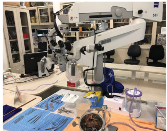
Fig. 4 Instructor's dissection workstation, equipped with a OPMI VARIO S88 microscope (Carl Zeiss SMT GmbH), surgical instruments, video system and a monitor (not shown).
