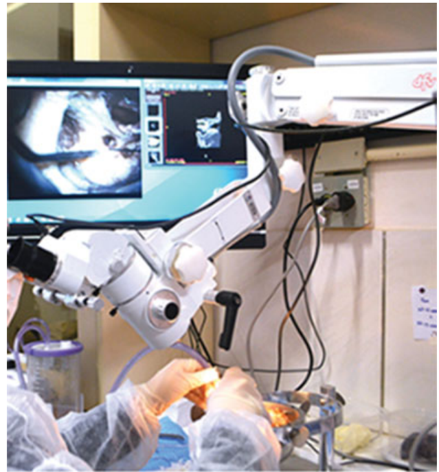
Fig. 3 Workstation with a MCM22 microscope (DF Vasconcellos Ltda.) and a computerized video system linked with a monitor. Screen shows simultaneously the video of dissection transmitted in real time from microscope next to a software window with CT images of the temporal bone being dissected. Abbreviation: CT, computed tomography
