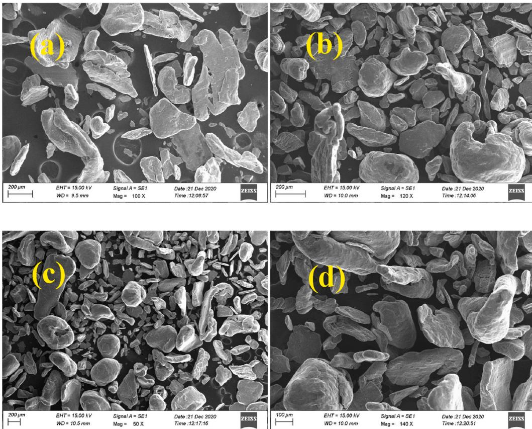
Fig. 4. SEM images of ball milled (a) Mg/3Al/3SiC (b) Mg/3Al/6SiC (c) & (d) Mg/3Al/9SiC powders.
