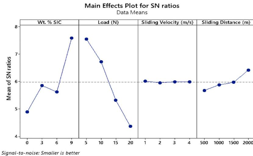
Fig. 8. S/N ratio plot of COF.
