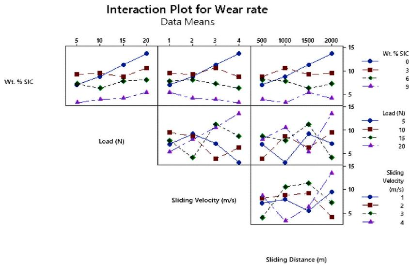
Fig. 12. Interaction plot for WR.
