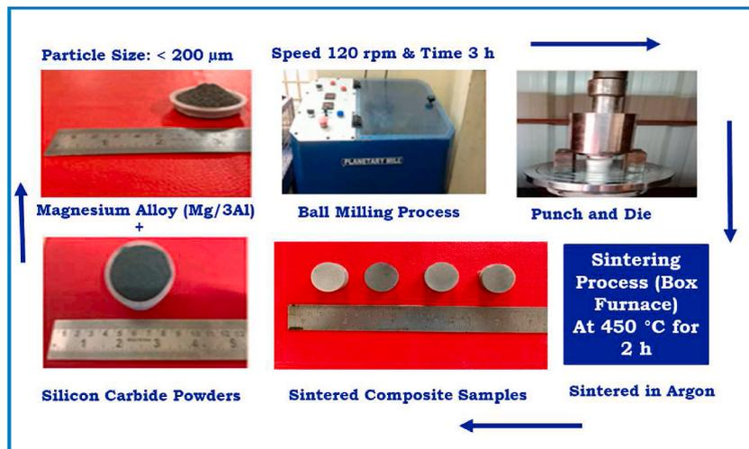
Fig. 1. Materials and experimental setup.
