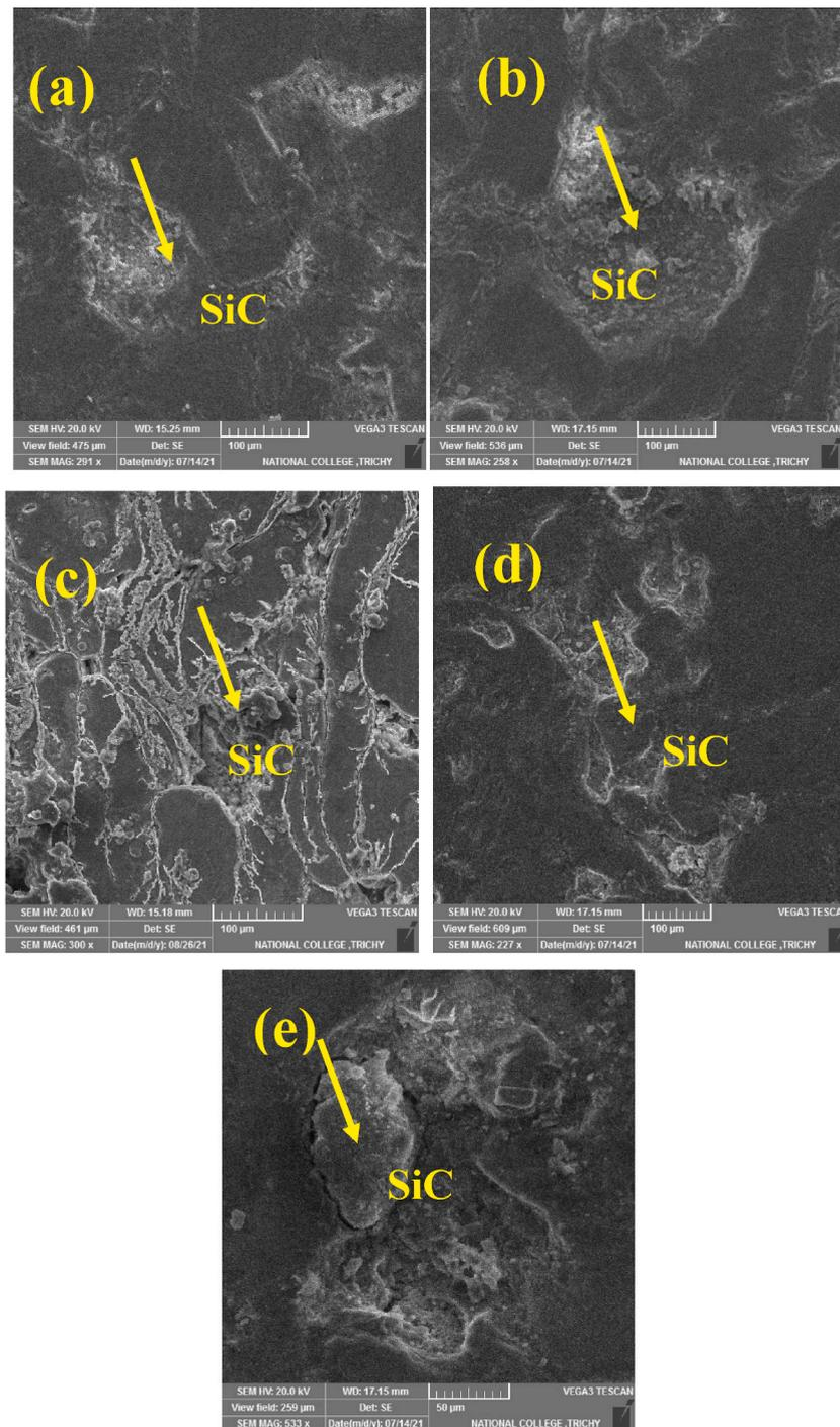
**Fig. 5.** SEM images of Sintered composites (a) Mg/3Al/3SiC, (b) Mg3Al/6 SiC, (c) Mg3Al/9SiC, (d) and (e) Mg3Al/9 SiC.
