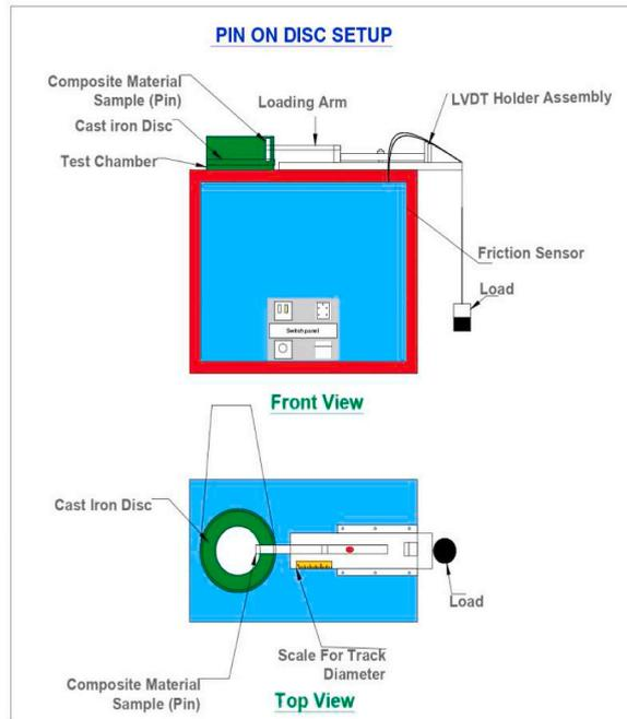
Fig. 3. Schematic of pin on disc.
