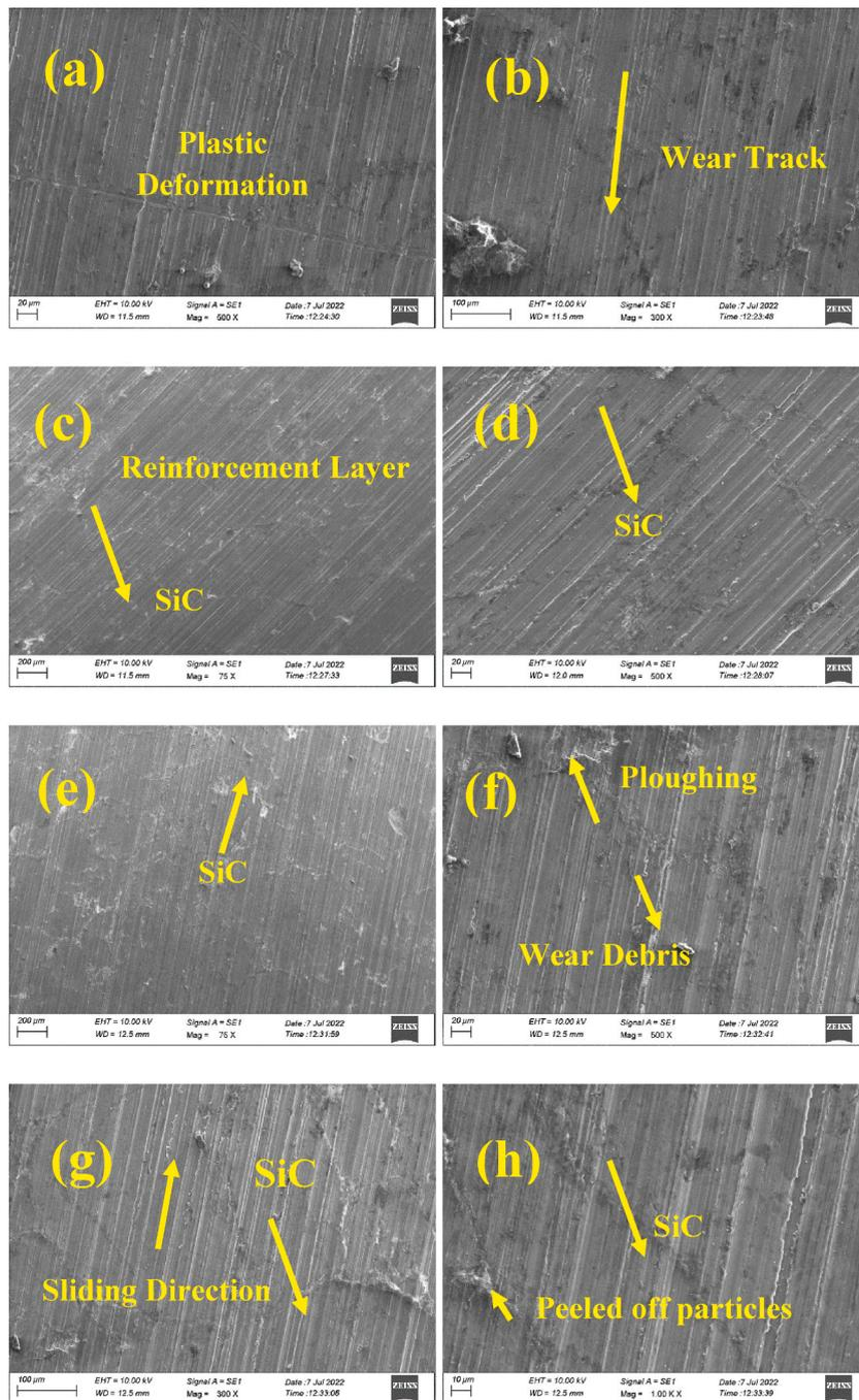
Fig. 16. (a–h) Worn surface analysis of Mg/3Al and its SiC reinforced composites.
