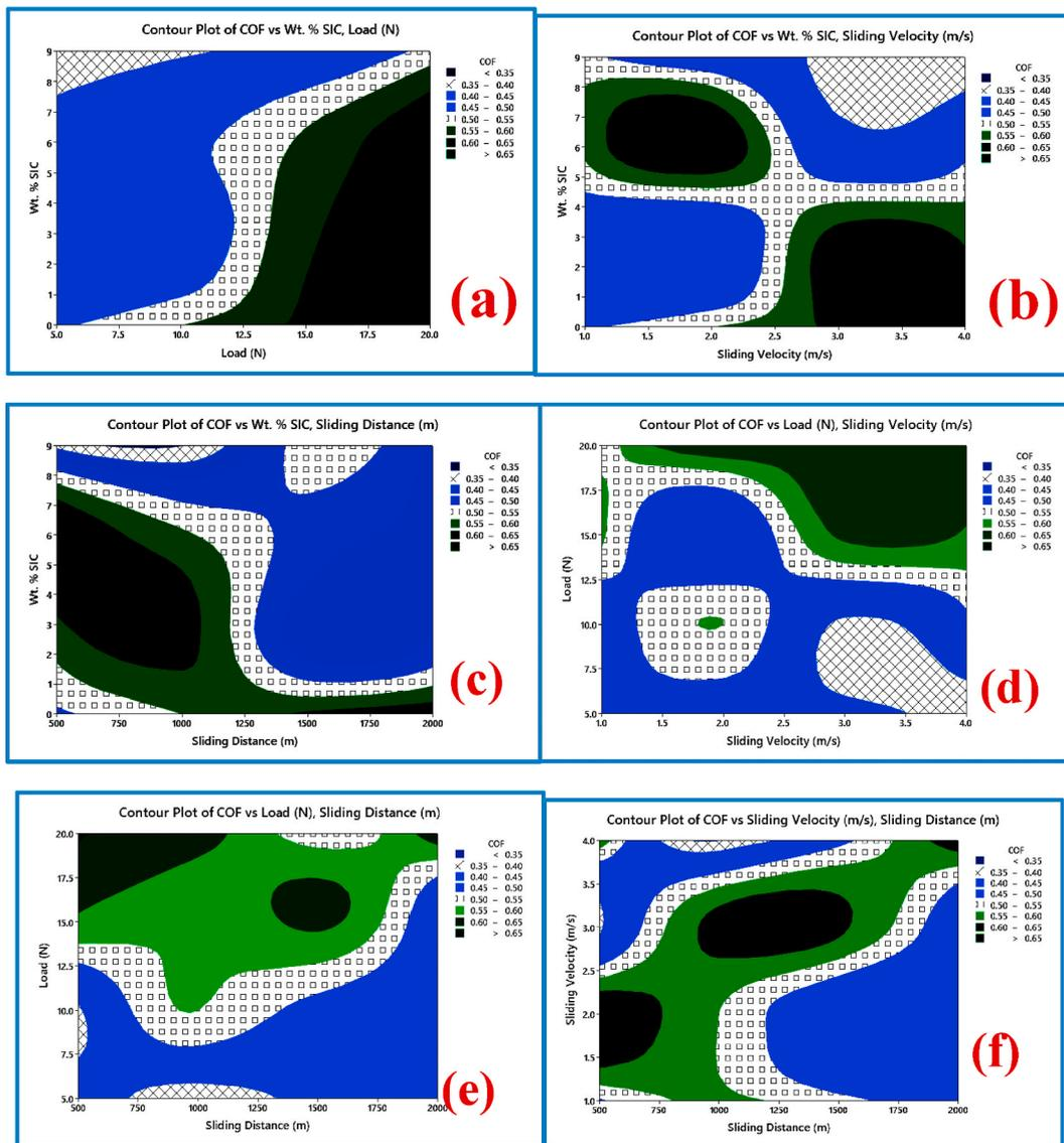
Fig. 11. (a–f) Contour plot for COF.
