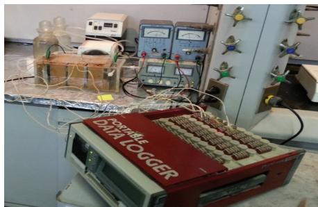
FIGURE 1: Coupled electrokinetics-adsorption experimental setup.
