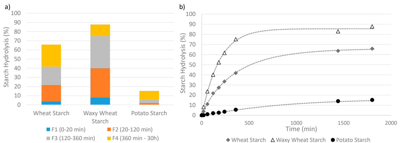
Figure 4. Two ways of analyzing degradability, applied to wheat starch, waxy (no-amylose) wheat starch, potato starch. (a) Identification of hydrolysable fractions of growing susceptibility to hydrolysis. The non-hydrolysable or Resistant fraction is the difference between the total amount of starch and the sum of all the digested fractions. Results are only for illustration as the data was not obtained from a standard in vitro digestion procedure. (b) Time-course measurements of the hydrolysis kinetics described by a fitted Weibull function.
