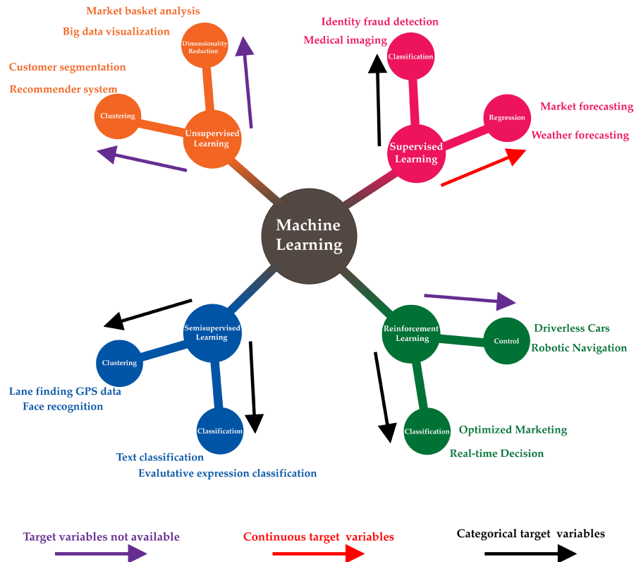
FIGURE 4 Machine learning. Different approaches to the learning process produce different machine-learning schemes. According to the number of features used to train the machine, one can obtain supervised learning (labelled data sets are used to train the machine), unsupervised learning (unlabelled data sets are used to train the machine), semi-supervised learning (a mix of labelled and unlabelled data sets are used to train the machine) and reinforcement learning (there are not data sets to train the machine). According to the quality of the target data (continuous or categorical), different tasks can be performed by the learning processes [Colour figure can be viewed at wileyonlinelibrary.com ]
