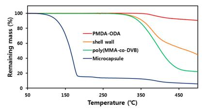
**Figure 11.** TGA thermograms of PMDA-ODA, the shell wall, poly(MMA-*co*-DVB), and the microcapsule. The shell wall sample was obtained by pressing the microcapsules between two slide glasses and drying.
