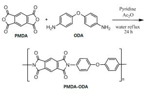
Scheme 1. Synthesis of PMDA-ODA oligoimide in water.
