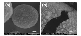
**Figure 9.** FE-SEM images of (**a**) *n*-hexadecane-loaded microcapsules prepared by oil-in-water Pickering emulsion templating and (**b**) the microcapsule shell wall.
