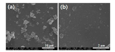
**Figure 3.** FE-SEM images of PMDA-ODA particles synthesized in water (**a**) before ultrasonication and (**b**) after ultrasonication for 30 min.
