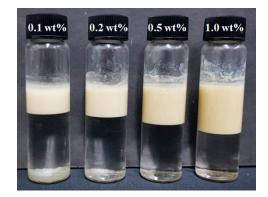
**Figure 5.** A photograph of PMDA-ODA particle-stabilized *n*-hexadecane-in-water Pickering emulsions prepared at different particle concentrations (0.1–1.0 wt %).
