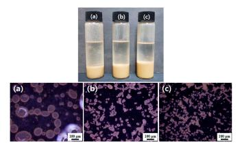
**Figure 8.** A photograph (**top**) and fluorescence micrographs (**bottom**) of water-in-decalin Pickering emulsions prepared at different PMDA-ODA particle concentrations: (**a**) 0.5 wt %, (**b**) 1.0 wt %, and (**c**) 1.5 wt %. The volume ratio of oil-water was 6:1. Fluorescence micrographs are provided for more clarity (excitation wavelength = 330~380 nm).
