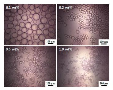
**Figure 6.** Optical micrographs of PMDA-ODA particle-stabilized *n*-hexadecane-in-water Pickering emulsions prepared at different particle concentrations (0.1–1.0 wt %).
