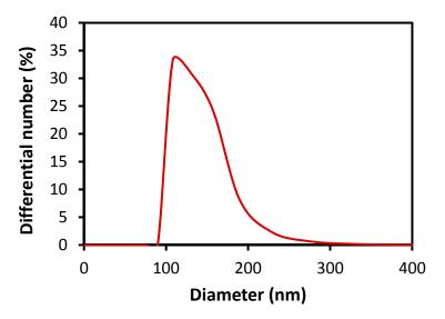
**Figure 4.** Size distribution of PMDA-ODA particles dispersed in distilled water (0.05 wt %) measured by dynamic light scattering (DLS).
