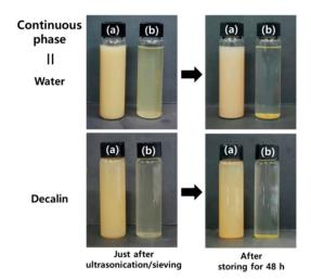
**Figure 2.** Photographs of dispersions of PMDA-ODA particles in water (**top**) and decalin (**bottom**) synthesized using (**a**) water and (**b**) NMP. The photographs were taken just after ultrasonication/sieving and after storing the samples for 48 h at room temperature.
