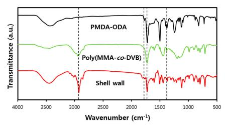
**Figure 10.** FT-IR spectra of PMDA-ODA, poly(MMA-*co*-DVB), and the shell wall. The shell wall sample was obtained by pressing the microcapsules between two slide glasses and drying.
