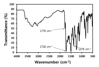
Figure 1. FT-IR spectrum of PMDA-ODA oligoimide synthesized in water.
