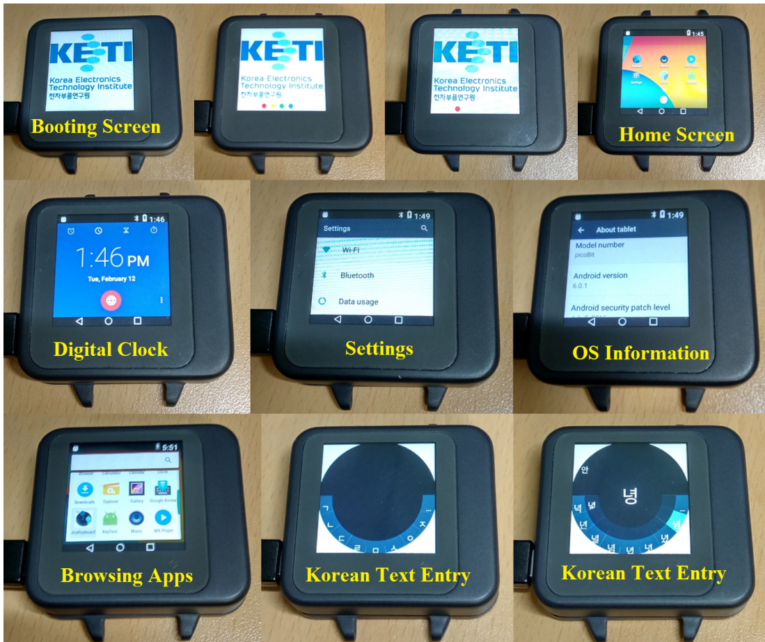
Figure 6. Final prototype with an enclosed case to resemble a smartwatch form factor.
