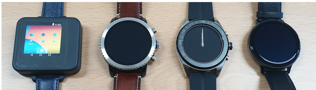
Figure 9. A side-by-side size comparison with commercial smartwatches (depicted from left to right, our prototype, Fossil Gen 3, LG Watch W7 and Samsung Galaxy Watch Active2, respectively).
