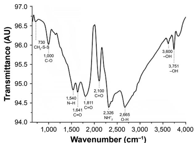
**Figure 7** FTIR spectrum of the biosynthesized AgNPs.
