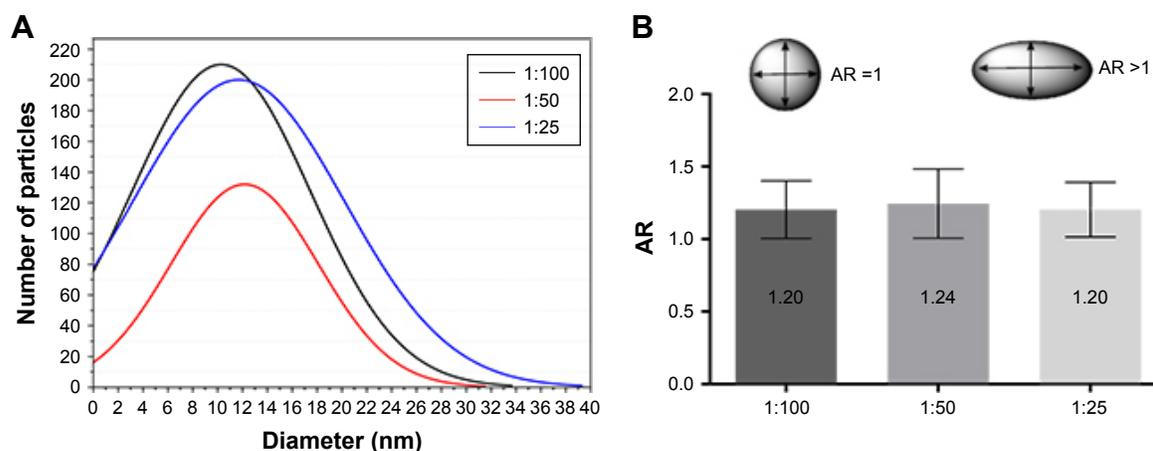
**Figure 6** Histogram of the diameter (**A**) and AR (**B**) of the AgNPs.
