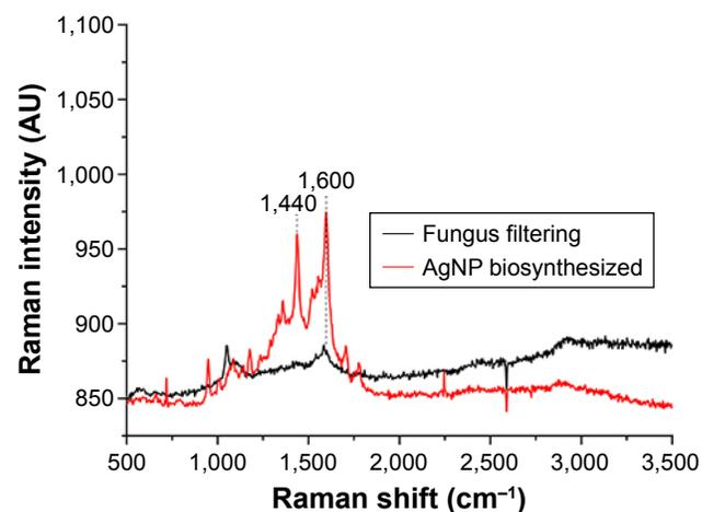
**Figure 8** Raman spectrum of the biosynthesized AgNPs.
