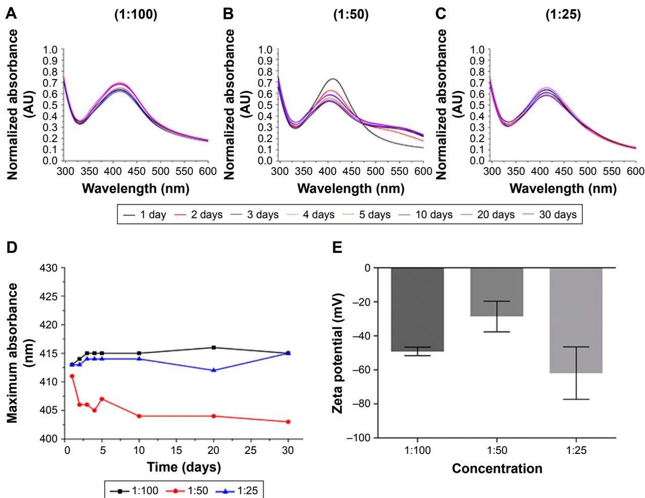
**Figure 2** UV–Visible spectrum as a function of reaction time of the aqueous solution of 1 mM AgNO<sub>3</sub> with the filtrate of fungal biomass, solution 1:100 (A), 1:50 (B), and 1:25 (C). (D) Mean maximum absorbency of the solutions. (E) Zeta potential of the AgNP biosynthesized in different concentrations of fungal filtrate.
