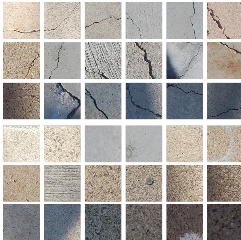
Figure 7. Representation of the images used to train labelling of crack images (the first three rows) and no-crack images (the last three rows).
