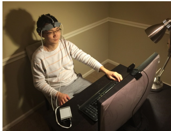
Figure 3. Experimental environment and participant wearing brain monitoring sensors.
