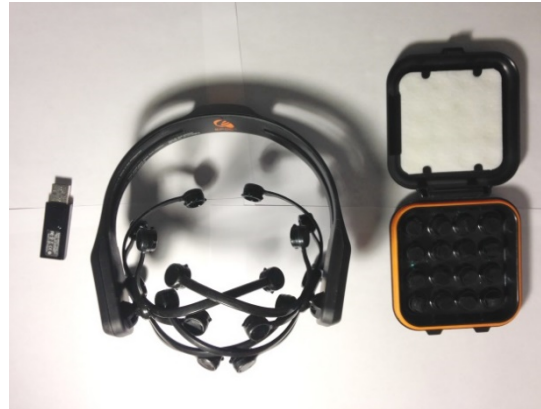
Figure 5. Emotiv EPOC headset: USB Dongle, EPOC headset, and electrodes [57].
