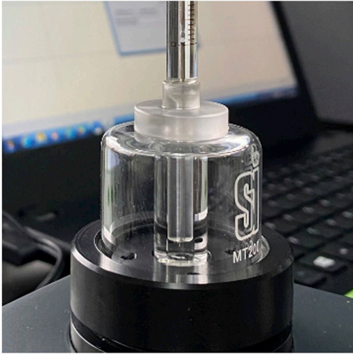
Figure 4. Add Saponin, Substrates or Inhibitors with a Microsyringe
