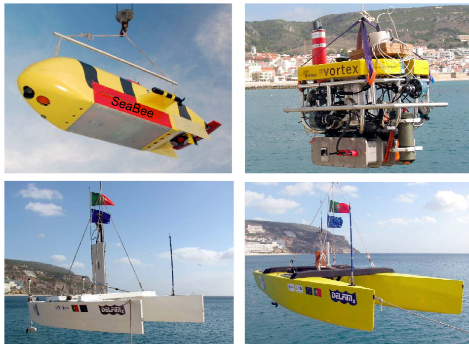
Figure 1. Heterogeneous vehicle used to demonstrate cooperative motion control during GREX trails at Sesimbra, Portugal.
