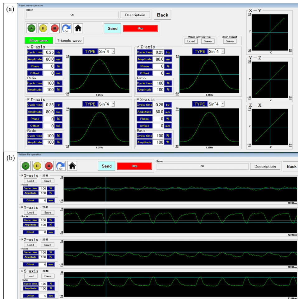
FIG. 2. Screen of the operating software for the four-axis moving phantom. The four-axis moving phantom generates (a) preset waves, such as sinusoidal and nth-power-of-sinusoidal patterns or (b) patient respiratory waves using pattern files, in a comma-separated values file format.
