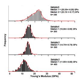
Figure 5. Mechanical data and distribution of Young's modulus obtained for sample 2, 3, 4 and 5.
