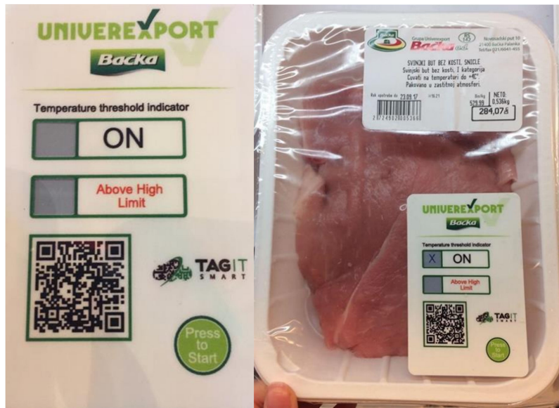
Figure 14. SmartTag with irreversible thermochromic sensor used in evaluation.
