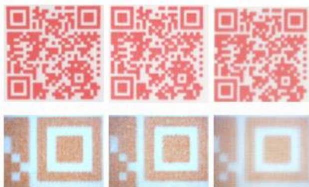
Figure 3. QR codes with 0.75 mm cell size printed with the thermochromic ink on different substrates: from left copy paper, label and photo paper. Pictures are taken with a camera ( above ) and with microscope ( below ).
