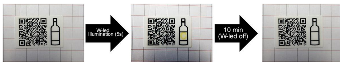
Figure 17. Activation of a SmartTag based on reversible W-LED-sensitive photochromic sensor.
