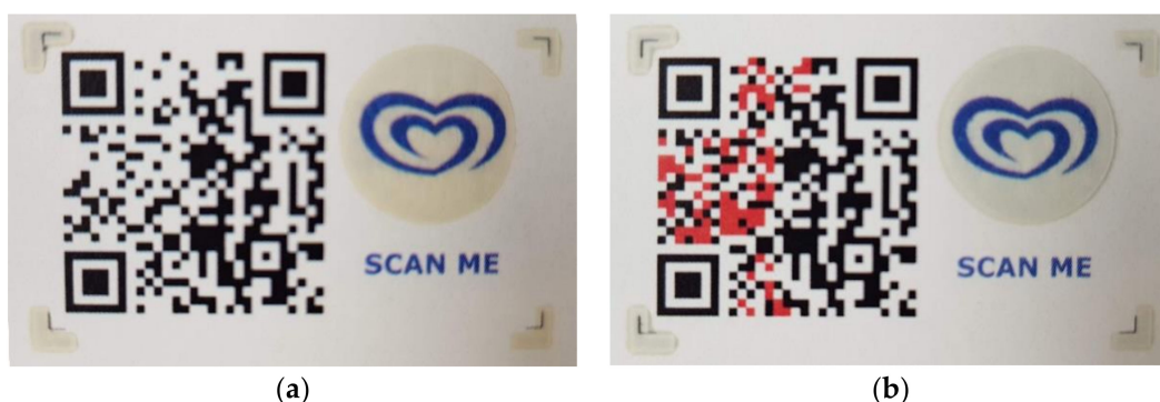
Figure 11. QR code before (a) and after (b) sensor state change encoded with two URLs with changed last two characters.
