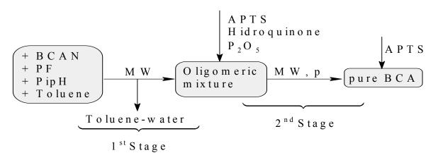
Figure 2. Direct synthesis of BCA assisted by microwave irradiation (MW).
