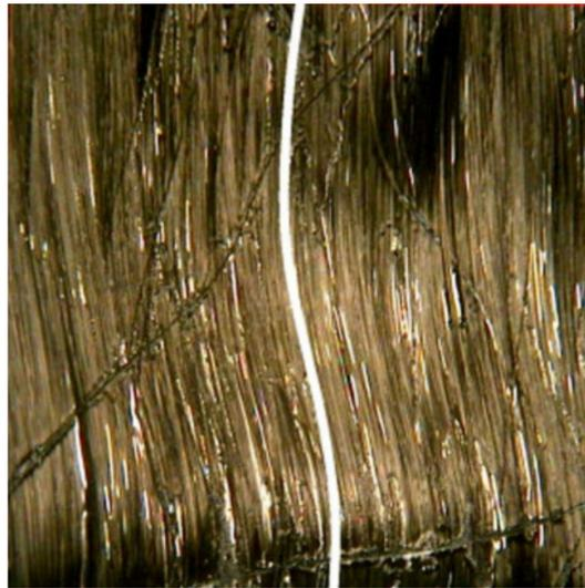
**Figure 5.** Level of fiber misalignment in a typical as-delivered unidirectional prepreg. Reproduced with copyright permission from Potter et al. [20].
