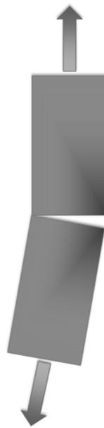
**Figure 4.** Stress distribution due to misaligned fibers.
