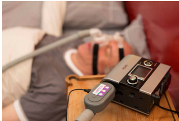
Fig. 1 NOWAPI ® stands on the patient circuit, at the output of the CPAP device. The diode indicator gives a traffic light feedback to the patient on the previous night CPAP treatment duration
