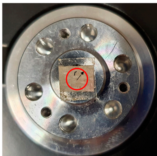
Figure 4. The spinning-cell setup. The substrate is mounted at the center of the rotating device and the laser is kept fixed at distance r from the rotation axis. During the SERS measurement, the laser track on the substrate follows the annular surface highlighted in red.
