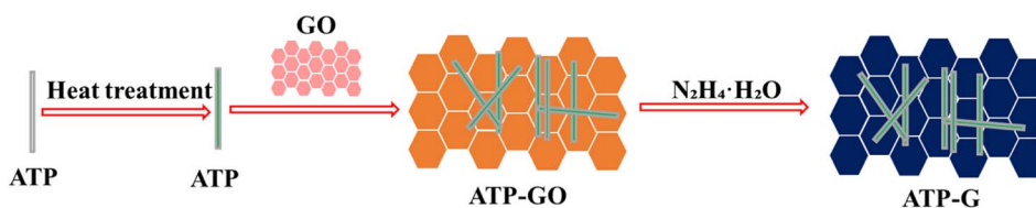
Fig. 1 Preparation process of the ATP–G nanocomposite.
