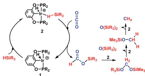
Scheme 3 Schematic representation of the hydrosilylation of  $\text{CO}_2$  to methane using the cationic Ir(III)-pincer complex proposed by Brookhart *et al.*
