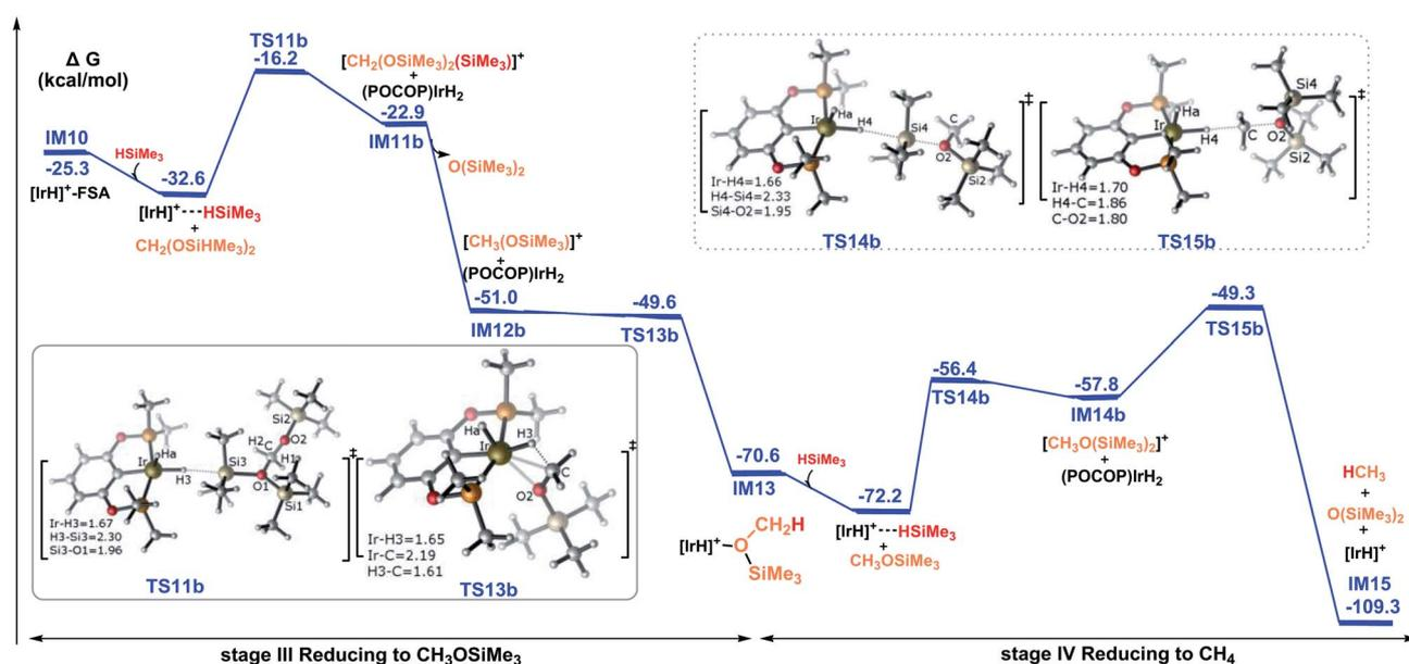
Fig. 6 Summary of the results for the hydrosilylation of bis(silyl)acetal to methoxysilane and methane, catalyzed by the cationic iridium complex *via* the ionic outer-sphere mechanistic pathways. The solvent-phase Gibbs free energies  $[\Delta G(\text{sol})]$  are in  $\text{kcal mol}^{-1}$ .
