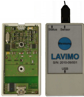
FIGURE 2. The sensor interface device (height 8.5 cm, width 4.5 cm, depth 2 cm). The microcontroller based sensor-PC interface device provides a USB connection for easy PC connection with an FTDI standard driver.
