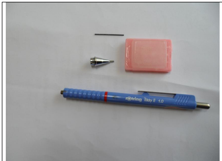
Figure 1 Mechanical pencil 1.0 mm used to manufacture the paraffin tissue punches.
