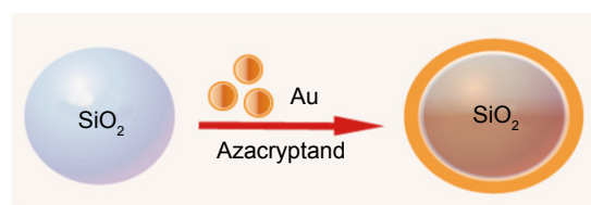
Figure 4 Schematic representation of synthesis of silica–gold nanoparticles.
