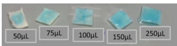
Fig. 1 Absorption test. Chondro-Gide matrices injected with different volumes of blue pigment solution.
