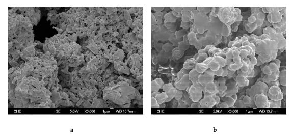
**Figure 7.** FE-SEM pictures of PP particles produced with homogeneous (**a**)  $Me_2Si(Ind)_2ZrCl_2$  and (**b**)  $C_2H_4(Ind)_2ZrCl_2$  catalysts at 0.2 wt% solution MAO concentrations and 55 °C at an agitation speed of 400 rpm.
