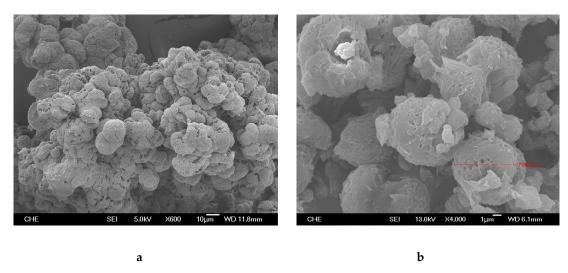
**Figure 6.** FE-SEM pictures of PP particles produced with  $C_2H_4(Ind)_2ZrCl_2$  at 0.4 wt% solution MAO concentrations and 55 °C at agitation speeds of (a) 400 rpm and (b) 100 rpm.
