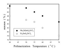
Figure 10. Effects of metallocene and polymerization temperature on [mmmm] of polymers produced.
