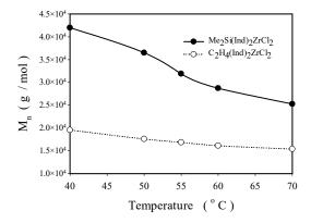
Figure 9. PP number average molecular weight vs. reaction temperature.
