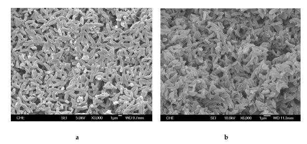
**Figure 12.** FE-SEM picture of PP particles produced with RHA-supported  $C_2H_4(Ind)_2ZrCl_2$  at (a) 40 °C, (b) 70 °C.
