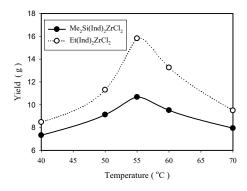
Figure 8. Influence of reaction temperature and metallocene on polymer yield.
