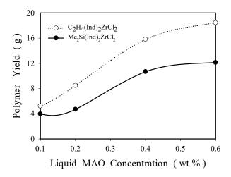
Figure 2. Effects of methylaluminoxane (MAO) concentration on polymer yield.
