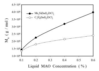
Figure 3. Influence of metallocene and MAO concentration on number average molecular weight (M<sub>n</sub>).
