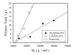
Figure 4. Relationships between polymer yield and number average molecular weight.
