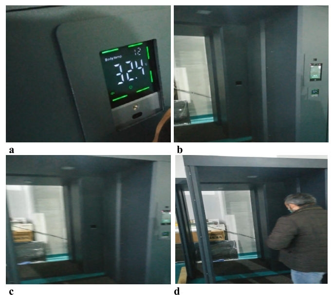
Fig. 25. a) StreamRobot gate face camera mode without face mask; b) Face-mask detection mode; c) StreamRobot gate deep learning scan for final verification to fog-cloud agents; and d) StreamRobot temperature mode.
