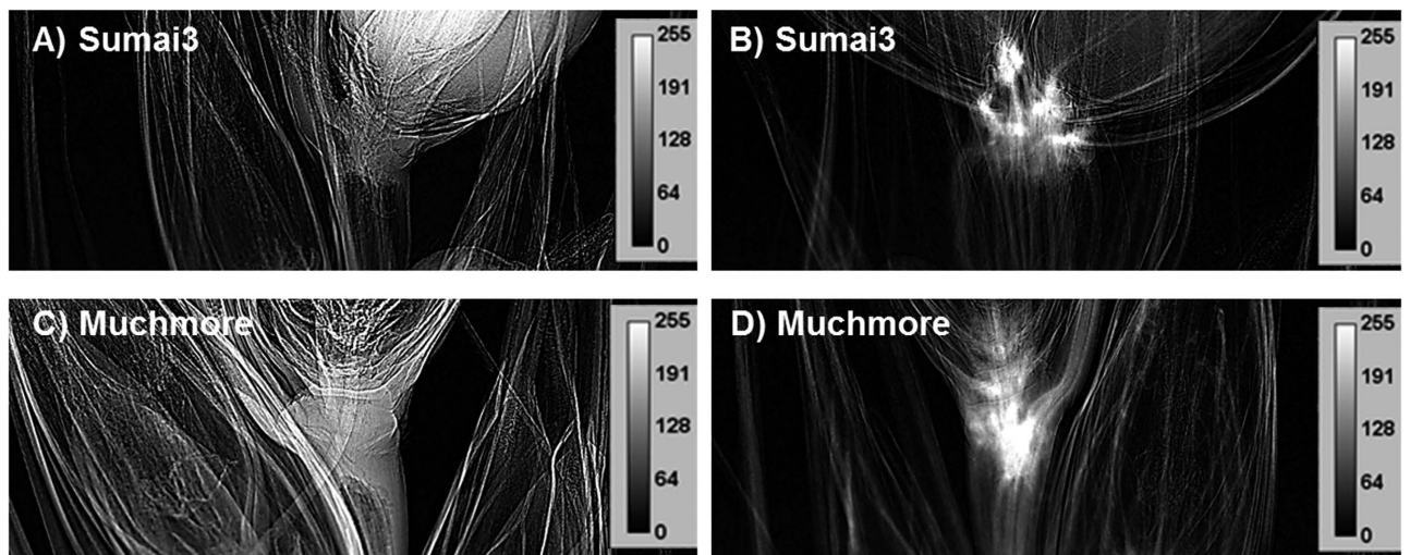
Figure 7. Use of contrast agents to study physiology of plants. The PCI of two wheat cultivar spikes recorded before (A) and after (B) introduction of iodine and water. The images were recorded at 18.0 keV (A,C) and 33.4 keV (B,D) using an effective pixel size of 8.75 \mu\text{m} .
