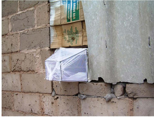
Figure 3. Window exit trap used for adult Anopheles mosquito surveillance, KwaZulu-Natal Province, South Africa.
