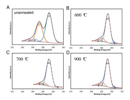
**Figure 8.** Comparison of the intensity of SP2 carbon peak intensity to C–O peak intensity from an (**A**) unannealed sample and after FA, at (**B**) 600 °C, (**C**) 700 °C and (**D**) 900 °C, for two hours.
