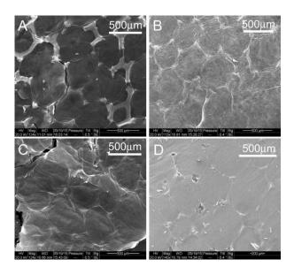
**Figure 4.** ESEM images of samples subject to FA at (**A**) 600 °C, (**B**) 700 °C, (**C**) 800 °C and (**D**) 900 °C, respectively.
