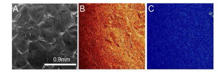
**Figure 6.** SEM image (**A**) and chemical map of carbon (**B**) and oxygen (**C**) distribution for an 800  $^{\circ}$ C annealed sample.
