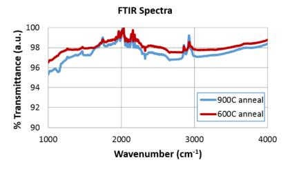
Figure 10. FTIR Spectra for thermal annealed samples.
