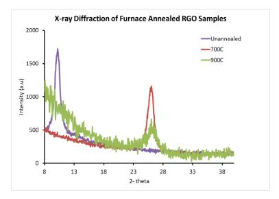
Figure 12. XRD data for furnace annealed samples.
