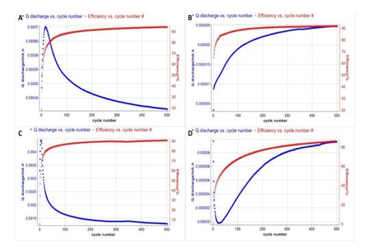
**Figure 14.** Constant current charging, discharging test for RGO-based electrodes with different annealing conditions: (**A**) 600 °C; (**B**) 700 °C; (**C**) 800 °C and (**D**) 900 °C. (The red line indicates efficiency vs. cycle number and the blue line discharge vs. cycle number).
