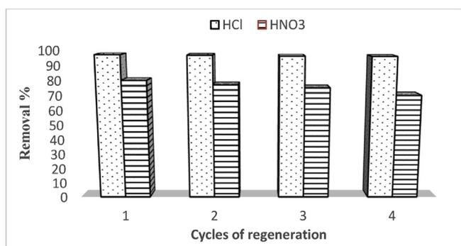
Fig. 13. Regeneration of  $Hg^{2+}$  ions from (Ag/Q)NPs composite.
