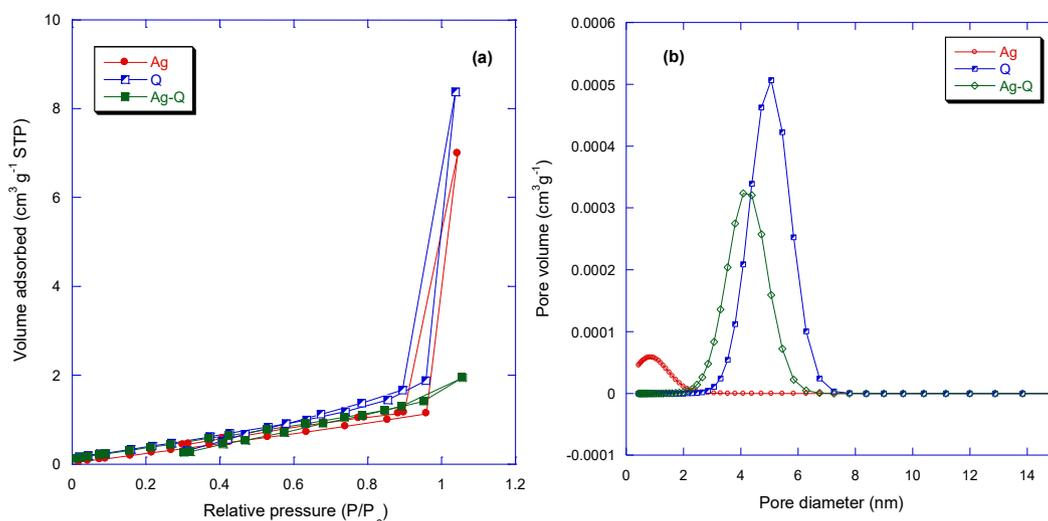
Fig. 2. (a)  $N_2$  adsorption-desorption isotherms and (b) the pore size distribution (PSD) curves of (AgNPs), quartz and AgNPs/quartz composite.
