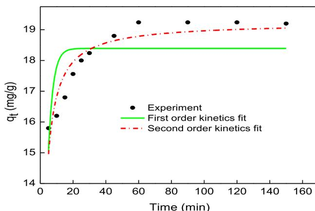
Fig. 9. Nonlinear fitting of Pseudo-first order and Pseudo-second order kinetics plots of  $\text{Hg}^{2+}$  ions adsorption onto (Ag/Q)NPs composite.
