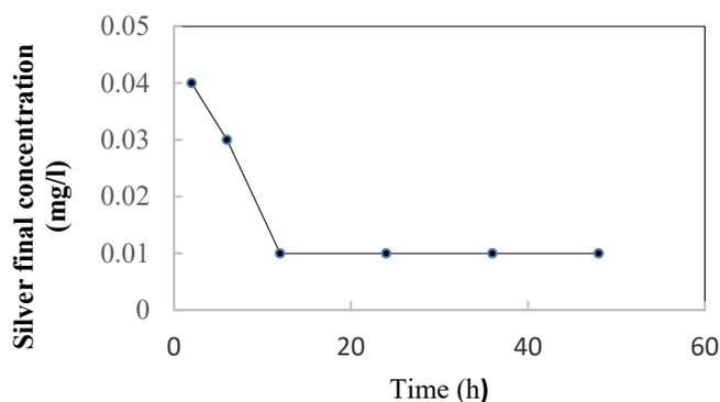
Fig. 12. Leaching test of Ag from (Ag/Q)NPs composite using distilled water.
