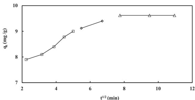
**Fig. 10.** Intraparticle diffusion kinetics of  $\text{Hg}^{2+}$  adsorption onto (Ag/Q) NPs composite (adsorbent dose: 0.5g, initial concentration:10 mg/l).
