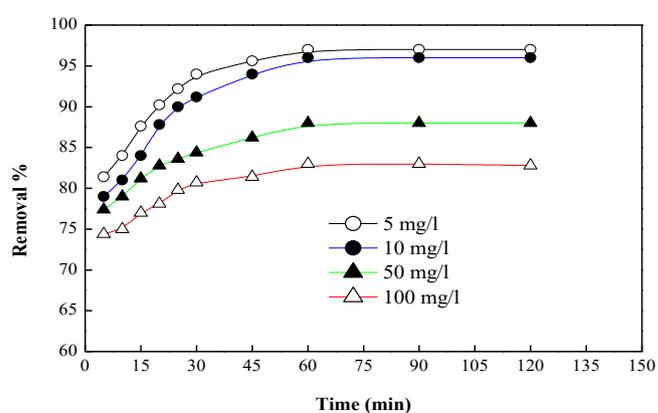
Fig. 5. Effect of contact time and initial concentration on the removal of  $Hg^{2+}$  by (Ag/Q)NPs composite (adsorbent dose = 1g, agitation speed: 200 rpm, initial metal concentration: 5,10, 50,100 mg/L).
