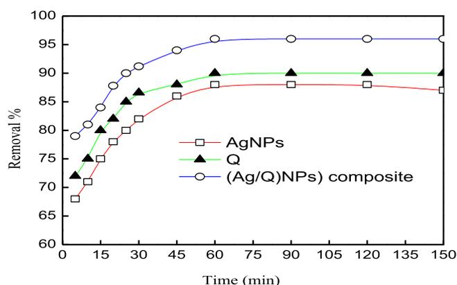
Fig. 4. Effect of contact time on the removal of  $Hg^{2+}$  by the prepared materials (adsorbent dose = 1g, initial concentration 10 ppm).
