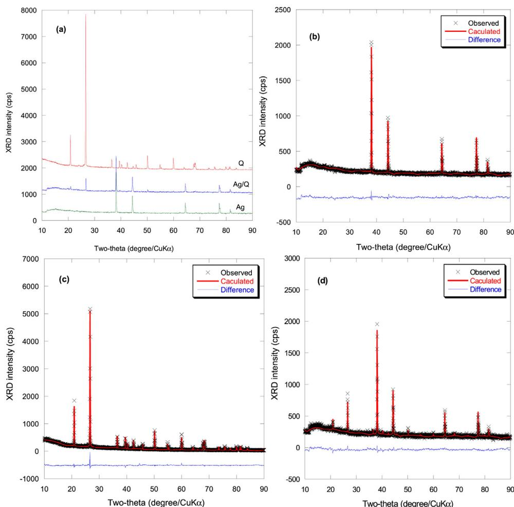
Fig. 1. (a) XRD pattern of AgNPs, Quartz and (Ag/Q)NPs composite and Rietveld refinements of XRD patterns of (b) AgNPs, (c) Quartz and (d) (Ag/Q)NPs composite.
