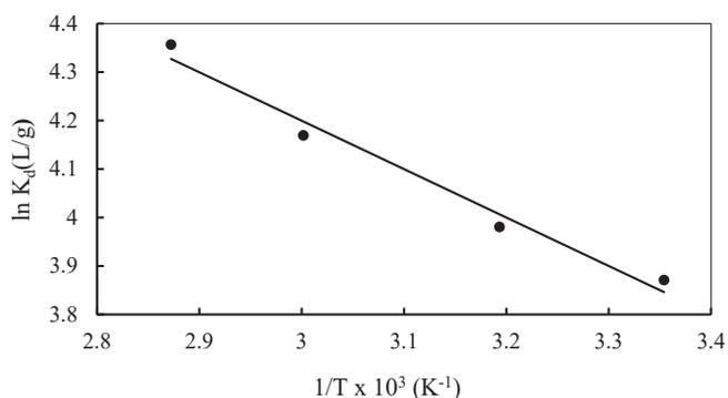
**Fig. 11.** Thermodynamic plot of  $\text{Hg}^{2+}$  adsorption onto (Ag/Q)NPs composite.
