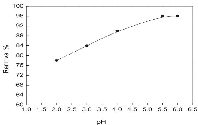
Fig. 6. Effect of pH on the removal of  $Hg^{2+}$  by (Ag/Q)NPs composite (amount of adsorbent: 1 g; agitation speed: 200 rpm, initial metal concentration: 10 mg/L).
