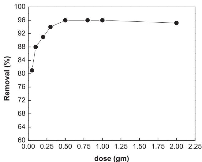
Fig. 7. Effect of adsorbent dose on the removal of  $\text{Hg}^{2+}$  by (Ag/Q)NPs composite (agitation speed: 200 rpm, initial metal concentration: 10 mg/L).
