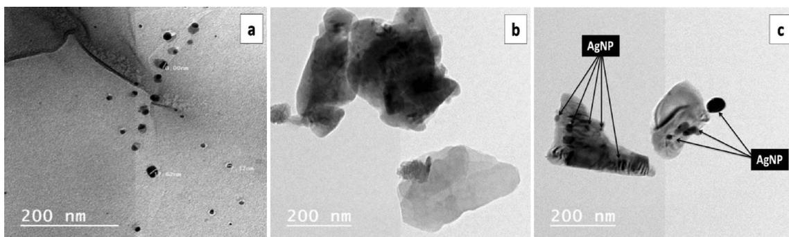
Fig. 3. TEM images of (a) AgNPs, (b) Quartz and (c) (Ag/Q)NPs composite.
