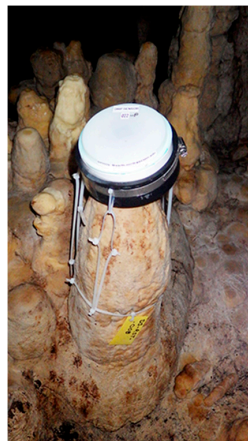
Figure 11. A drip-sensor tethered by cable ties to the top of a stalagmite, at a slight incline to prevent water accumulating on the surface.
