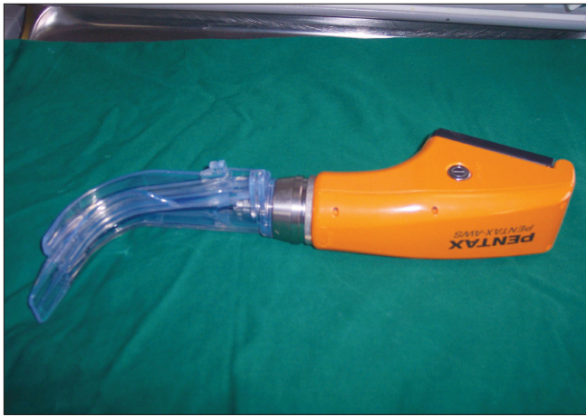
Figure 1: Assembled pentax video laryngoscope
