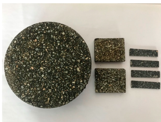
Figure 1. Asphalt mortar samples.
