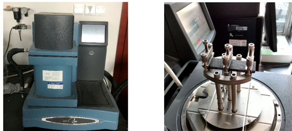
Figure 2. DMA instrument and dual cantilever clamp.
