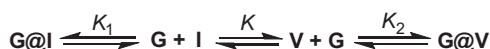
Fig. 5 Conformational interconversion and complexation equilibria. K_1 and K_2 are the association constants of a guest with conformers I and V, respectively; K is the equilibrium constant between the two conformations.
