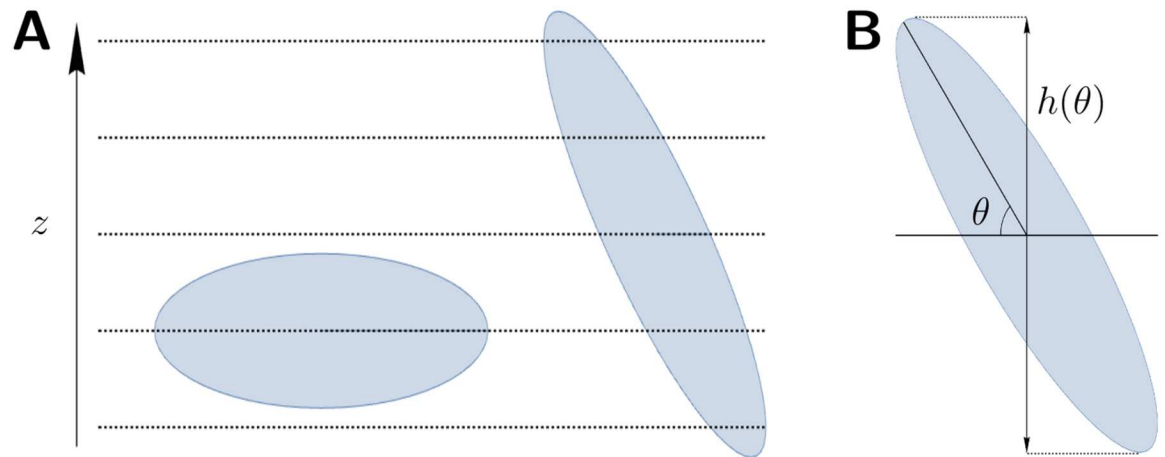
Fig 18. The effect of nuclear orientation on sample probability. A: Comparison of the sectioning of two nuclei at different angles to the plane. The nucleus lying within the plane is only sampled once, whereas the nucleus which is more vertical is sampled multiple times in sectioning. B: The height function h of angle \theta . The value of h(\theta) is the difference in height between the highest and lowest points on a nucleus at angle \theta .
