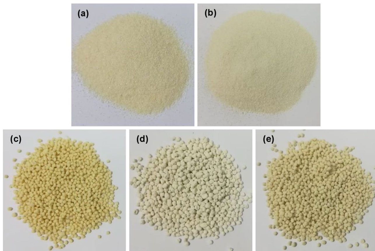
Figure 1. Physical characteristics of (a) chitosan standard, (b) chitosan powder (CP), (c) chitosan beads (CB), (d) chitosan beads mixed ZnO (CZB), and (e) chitosan beads coated ZnO (ZCB).
